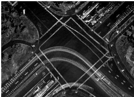
Fig. 4. The two channels of our probabilistic maps. In (a) we see the average infrared reflectivity, of brightness, of each cell. The innovation of this paper is to also consider (b), the extent to which the brightness of each cell varies. Note that the trails of the passing vehicles are much more prominent in (b).
