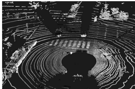
Fig. 3. Without calibration (a), each of the 64 beams has a significantly different response to reflectivity values. After calibration (b), the beams are much better matched.
